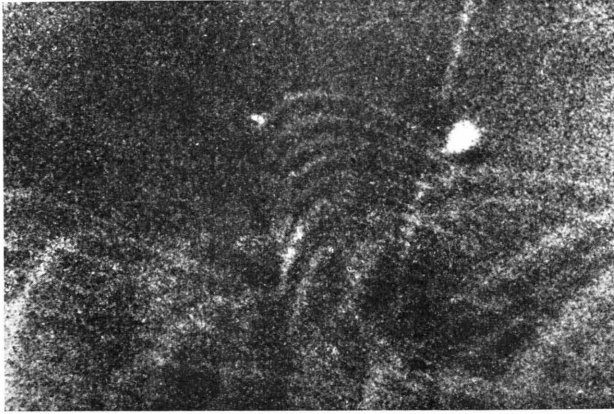
Fig. 6. Dislocation loops on the boundary between dislocation-free and distorted part of silicon specimen III. Borrmann's case topography on a double crystal spectrometer [ R(2\bar{2}0) diffraction, the area shown on the figure is 1.23 \text{ mm} \times 1.88 \text{ mm} ].
